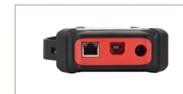
LAN/WAN Port, Data I/O port & DC-IN Power Jack
