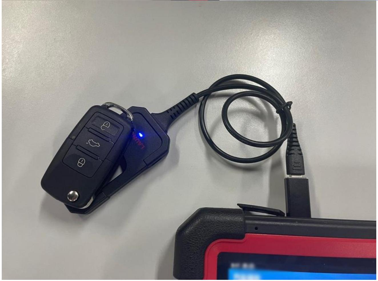
3. After the remote control is successfully generated, enter the [Set type of super chip] menu to generate the corresponding key chip.
