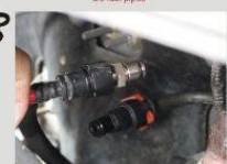
Connect the two adapter connectors to the fuel pipes.
